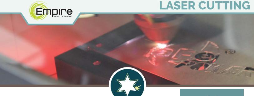
Empire's compact laser cutter has fast rise time, high peak power pulse (3x above the average power) and excellent beam quality for high quality, clean cutting. This pulsed, sealed laser has capabilities for cutting aluminum, wood, adhesives, and more. It is efficient and has low operating costs. The high peak power, square pulse, and excellent mode means that it quickly vaporizes material and produces a clean narrow cut. Think outside the box with laser cutting!
