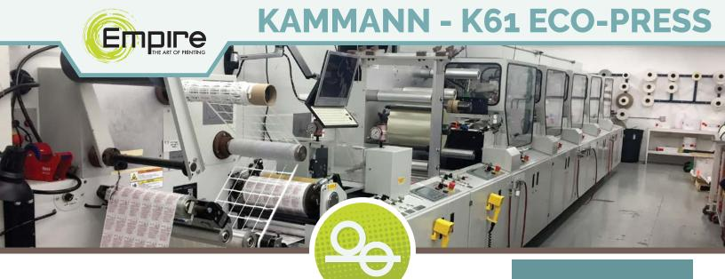
Empire offers the convenience of roll-to-roll labels with the outdoor-durability of screen printing. The Kammann K-61 EcoPress is the first screen press that uses a UV LED ink curing system, making it the most economically sound and environmentally friendly screen printing press on the market.
